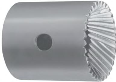
Outside Deburring Cutters are designed with shear-type cutting teeth to eliminate burrs on diameters of tubes and rods. One tool can handle various parts, may be reground, and can be provided in carbide.
