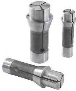
An **Emergency Collet** may be used when a standard collet is not in your current inventory. It can be machined to the desired bore size and used until a hardened collet arrives.
