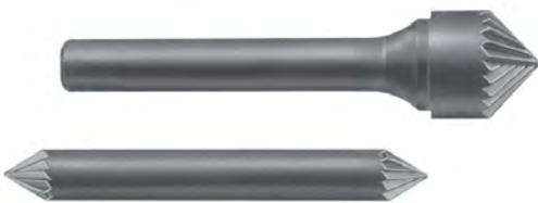
All carbide Inside Deburring Cutters are designed with a pointed nose. Tools with a head diameter measuring 3/32" thru 1/4" are made of solid carbide and are double ended. Inside Deburring Cutters with a head diameter measuring 5/16" thru 1" have solid carbide heads brazed to hardened alloy precision ground shanks.
