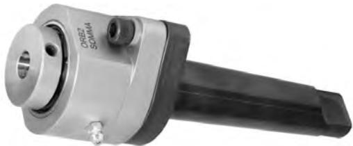
The broach tool holder is designed with a live spindle which holds the cutting broach at a 1° angle. This design creates a wobble effect on the cutting broach which reduces the cutting profile and thus minimizes the required force that is needed to produce the internal shape.
