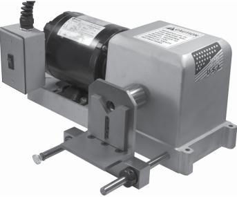
The STC-TAP-ER has a double disc friction drive that reverses rotation instantly by the application of forward or backward hand pressure on the part being tapped. The friction discs are driven by a Heavy Duty Tapered Cone Drive Collar mounted on the motor shaft. The maximum spindle speed is 300 RPM.
