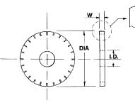
These high speed steel circular deburring tools fit the slotting attachment of B&S Screw Machines and Swiss Machines and remove cut-off burrs from the back end of the part completely, smoothly and uniformly.
