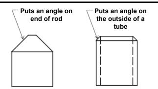
Works well on both tubing and rods
